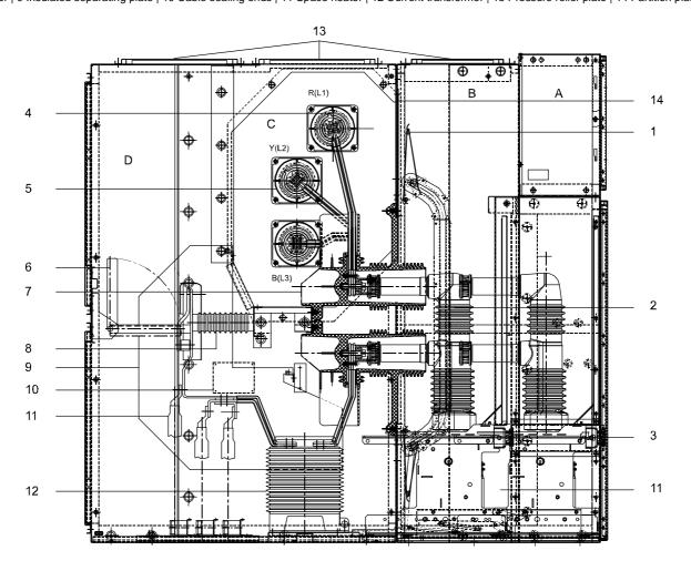
The basic structure of the switchgear panel comprises the panel itself and withdrawable part with circuit breaker.
