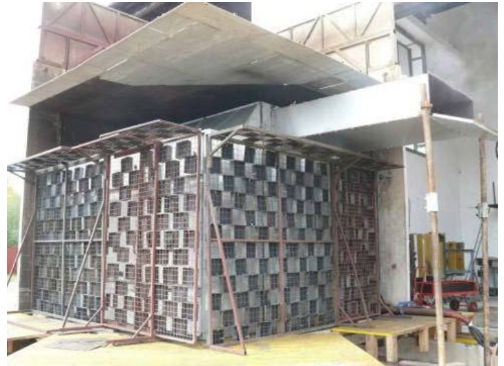
UniGear ZS2 during internal arc test
