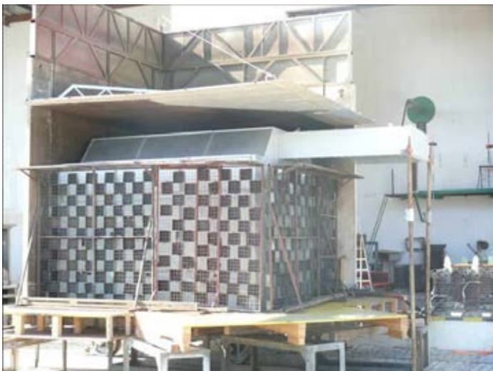
UniGear ZS2 during internal arc test
